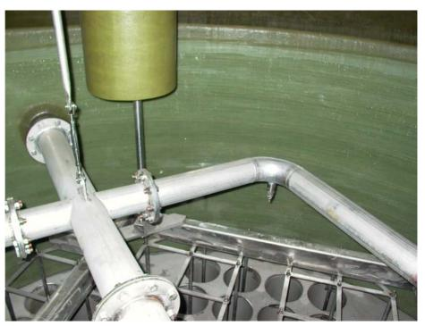
Figure – Interior from wet electrostatic precipitator.
